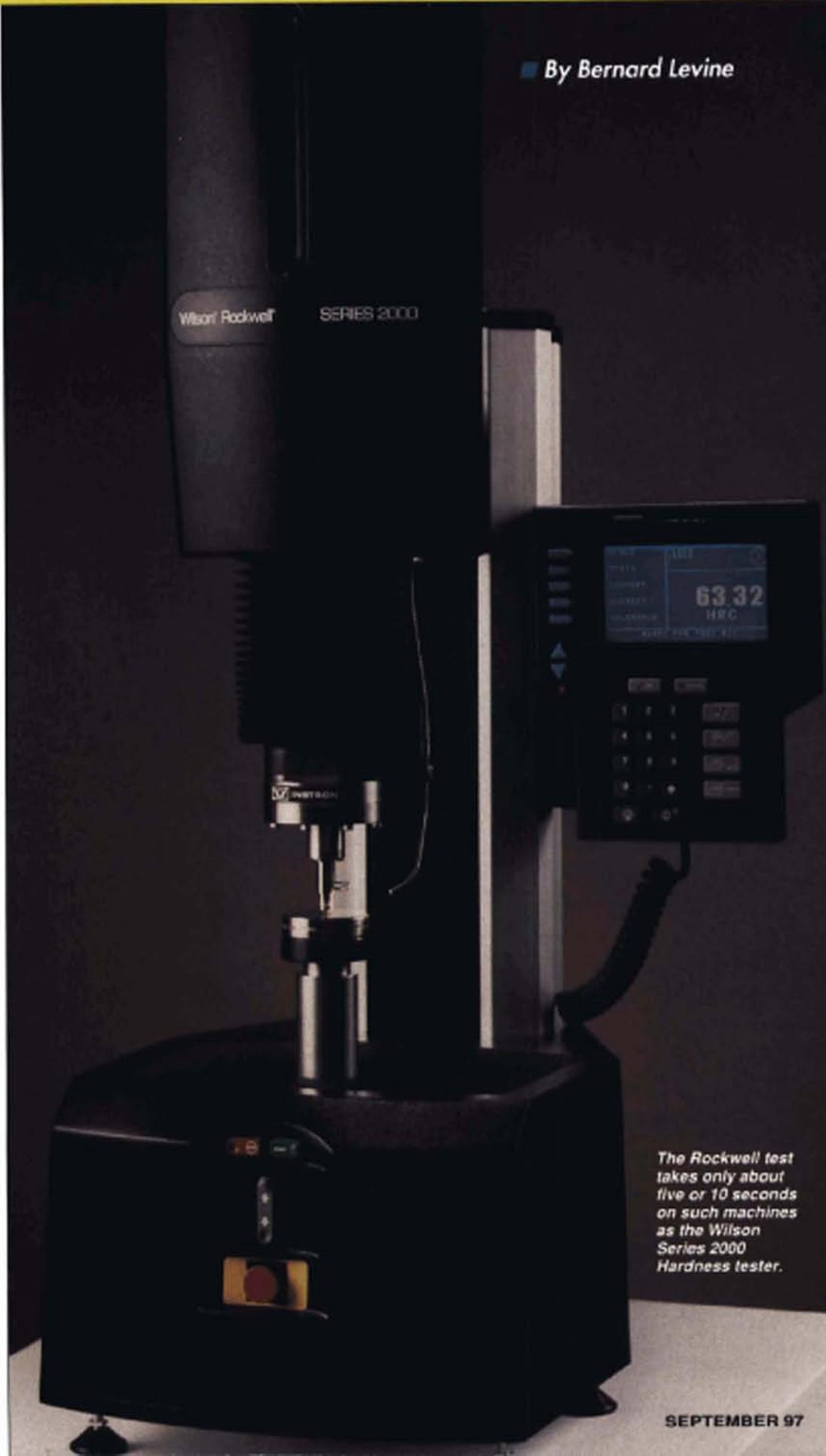
*The Rockwell test takes only about five or 10 seconds on such machines as the Wilson Series 2000 Hardness tester.*
